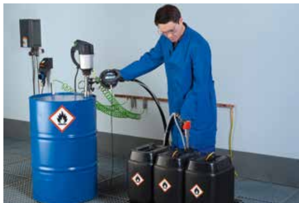
Semi-automatic canister filling in Ex-zone 1.
